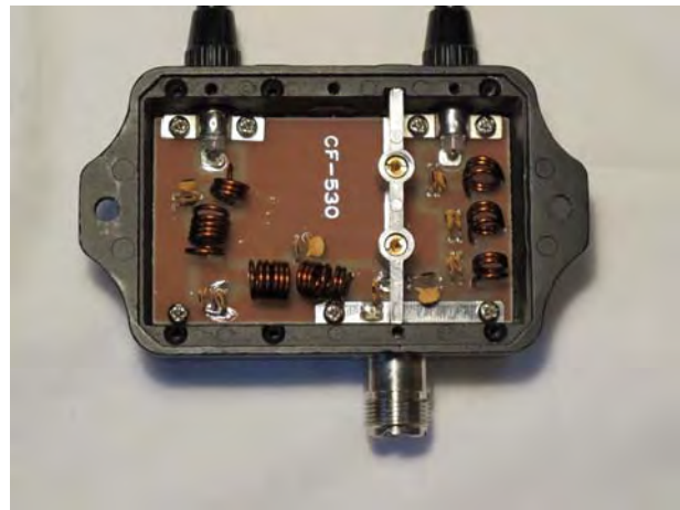
Fig 8 : Internal view of the ‘600watt’ rated unit
